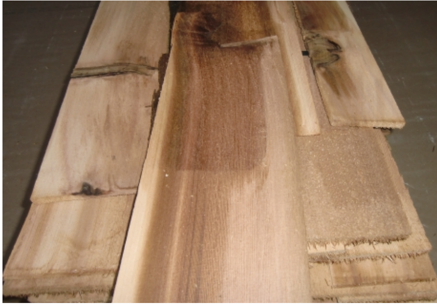
Unpermitted knots within a bundle
