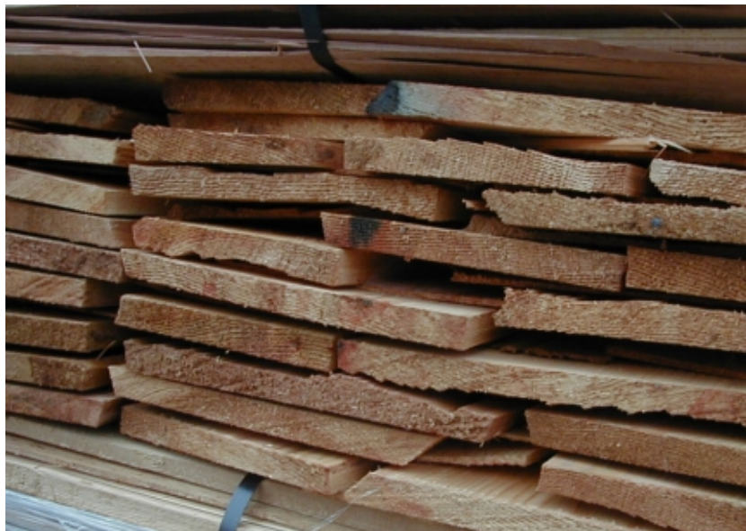
18" x 5/8" Tapersawn Shakes. Bundle was opened and when graded was found to contain excessive narrow shakes.
